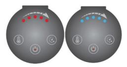
Constant temperature mode: adjustable temperature range 45 °C -65 °C, default temperature 65 °C, the 1st red light is 45 °C, each red light lit later increases by 5. As shown in following picture
