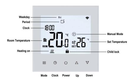
The current room temperature is displayed on the left of the screen and the desired room temperature on the right.
